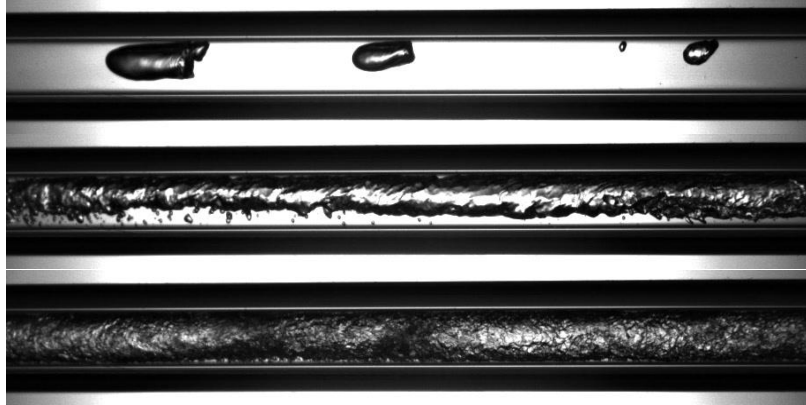
Figure 4. Flow structures of R1233zd(E) in 3mm horizontal pipe under saturation temperature 83°C, saturation pressure 0.71 MPa, reduced pressure 0.2, and mass velocity 1000 kg/(m 2 s)
