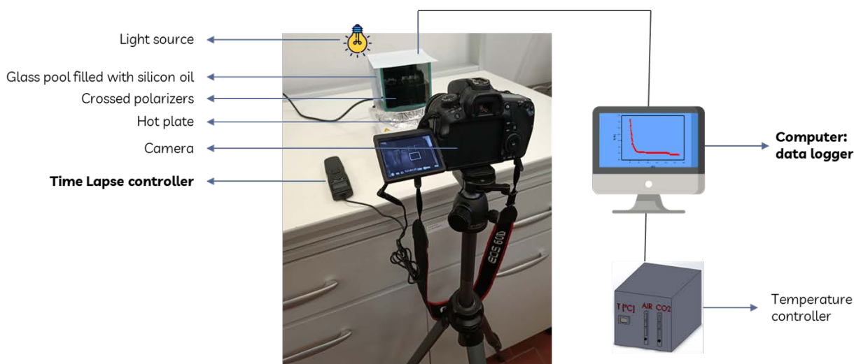
Figure 1. Visual inspection set-up.
