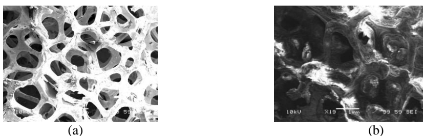
Figure 1. Samples SEM image (a) copper foam (b) paraffin/Cu-foam composite ( \epsilon = 96.1\% , \omega = 40 PPI)
